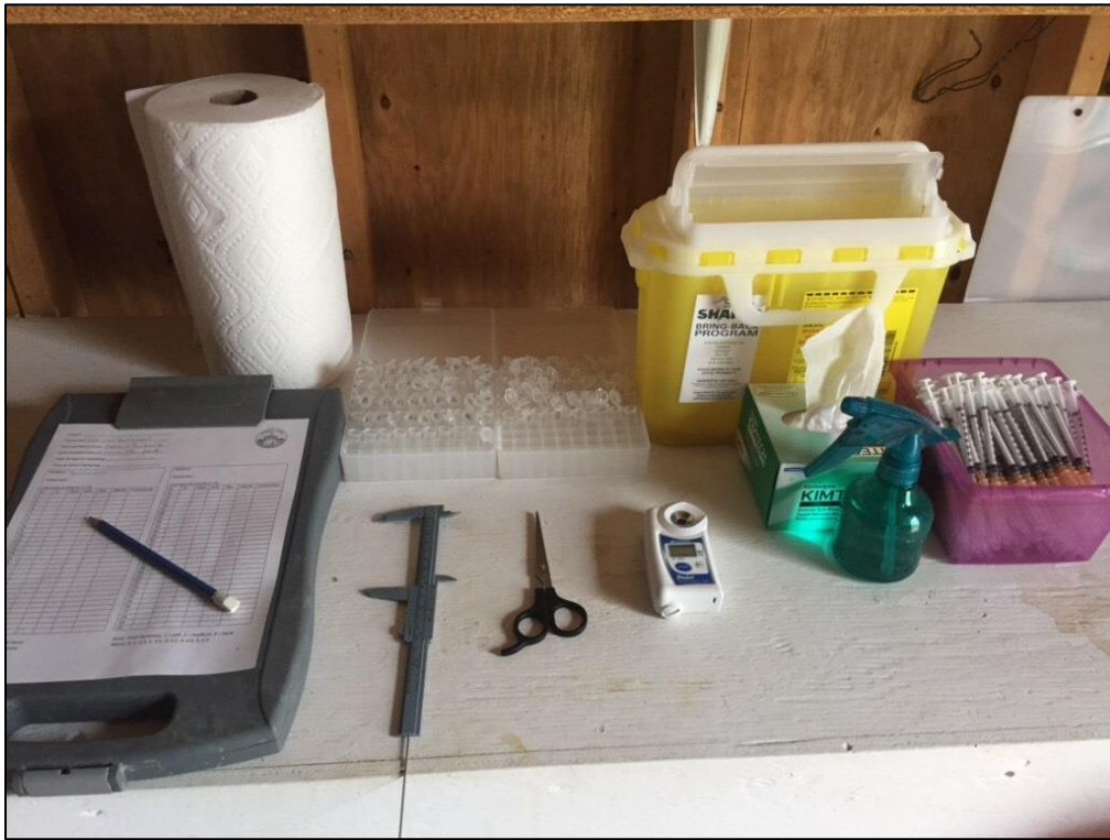
A typical sampling set up including: data sheets, carapace measuring tool, Brix Refractometer, syringe and needle (and disposal), vials for transporting pleopod sample.
